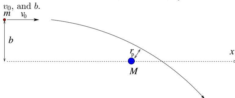
To do this, first note that through conservation of energy, you can find an expression relating the *magnitude* of the velocity  $v(r)$  at any radius  $r$ , in terms of  $r$ ,  $M$ , and  $v_0$ .
